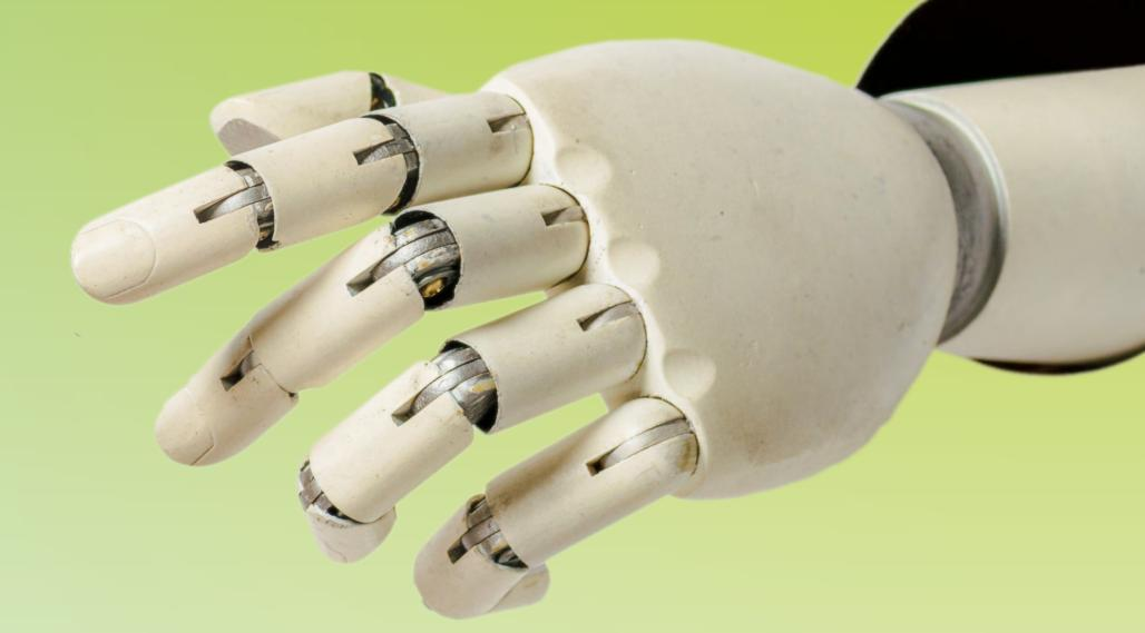
Create a working model of a robot hand. When finished, the fingers on the model will be controlled by pulling on the strings. The mechanism of this robot hand mimics the pulley system used in many robots in factories today!
